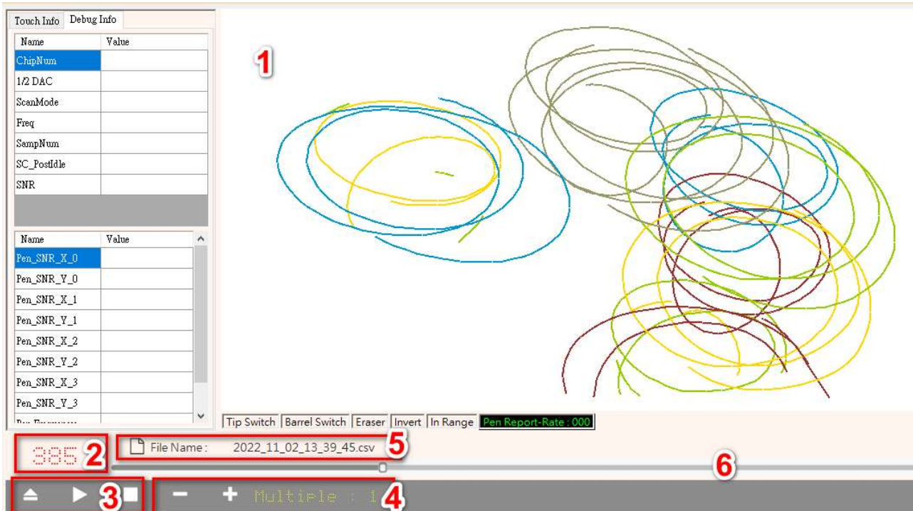
Fig 3-18 The thickness of the track changes according to the pressure when using the stylus
